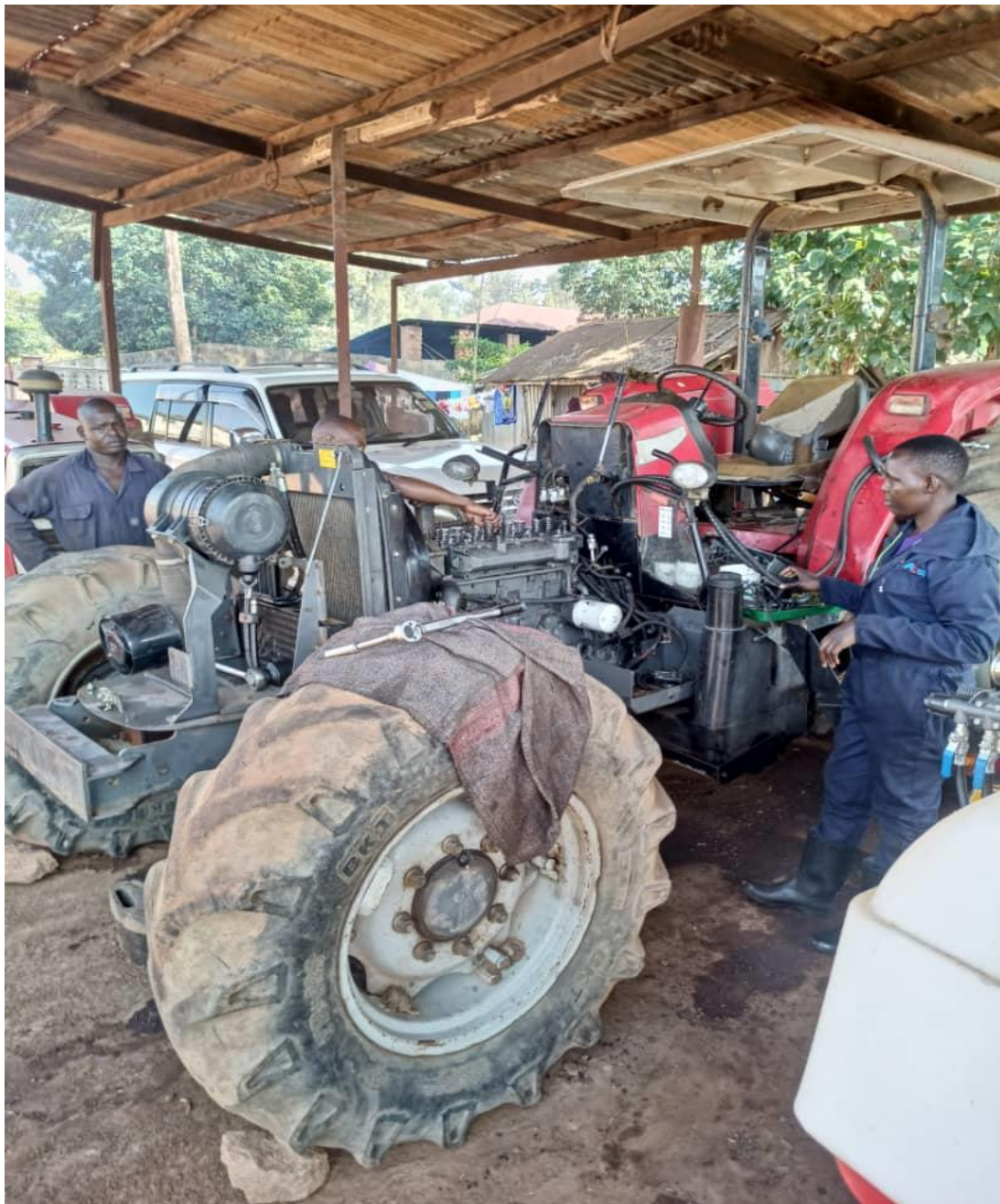
Figure 20: Tractor UG0251U being tested after engine overhaul at our Tractor maintenance unit Luzira
